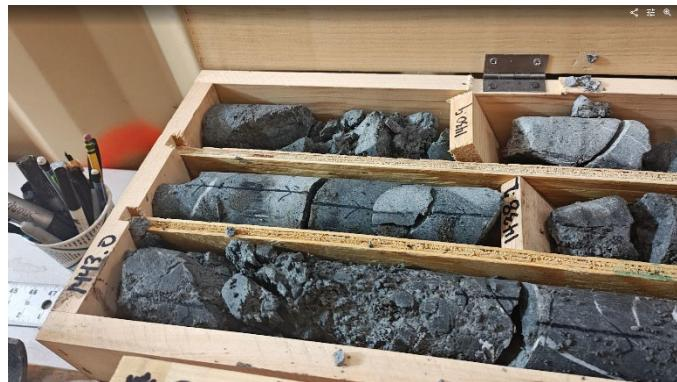
*Samples from horizontal rock coring, taken during geotechnical drilling completed in January 2026. The data collected will help shape design and construction of the Last Chance Grade bypass tunnel.*
