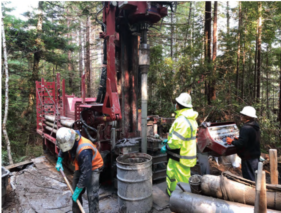
Mid-Roto Sonic 50K track rig on Green Diamond property. D-20-002 (B-40) Gregg Drilling
