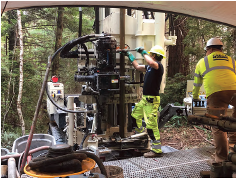
Geoprobe 3230 mud rotary rig on Green Diamond property. D-20-002 (B-40) Gregg Drilling
