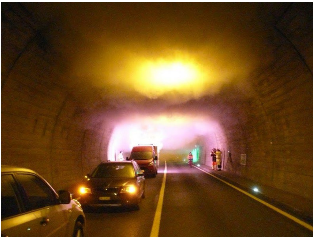
Figure 14. Smoke Stratification Under Controlled Flow Conditions in a Bidirectional Road Tunnel
