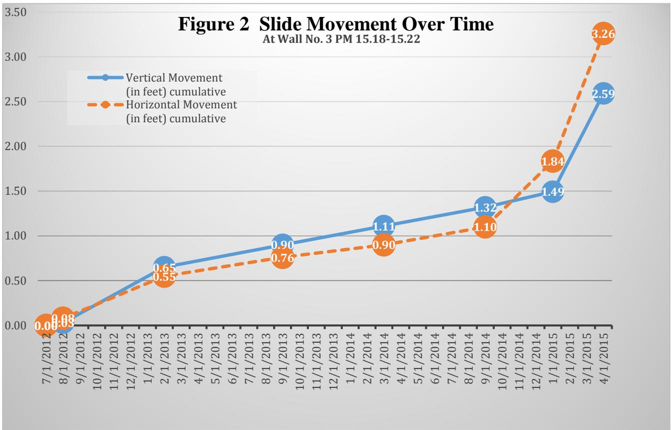
Figure 2 is a graphical representation of slide movement over time. Monitoring began in July of 2012 when sensors and a survey network were installed during the construction of a retaining wall. Movement is measured in feet; vertical movement is downwards, and horizontal movement is westwards.
