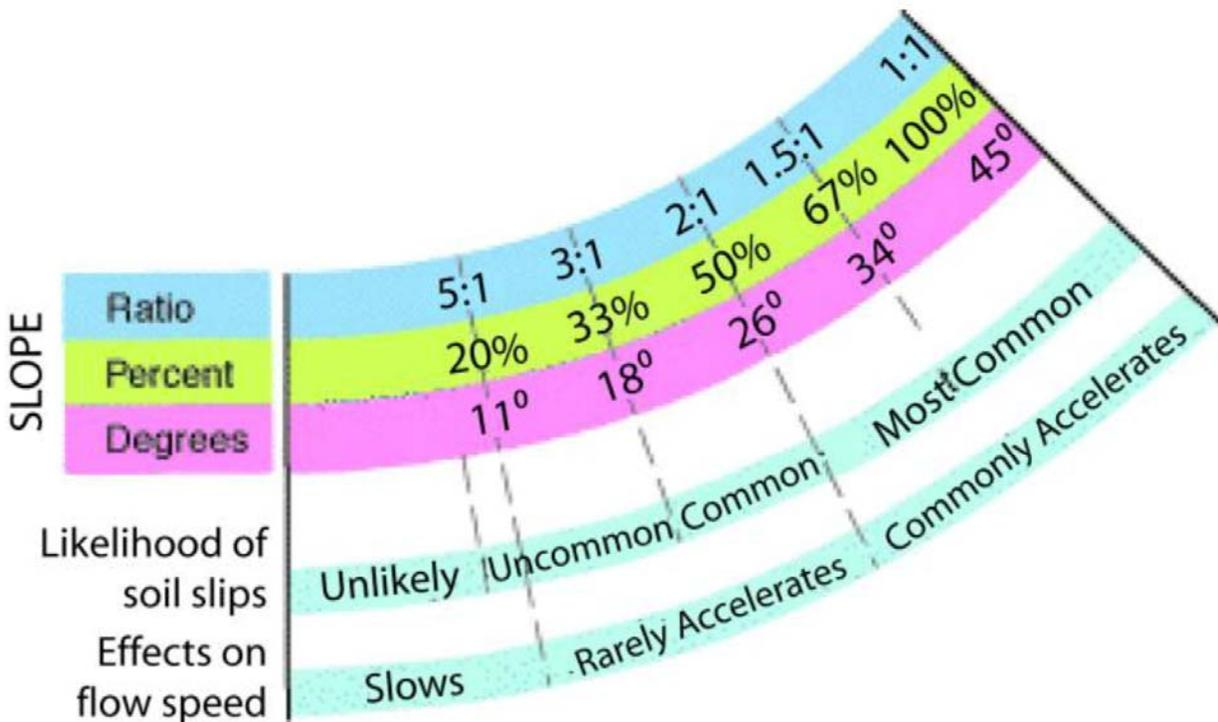
Figure 819.7E Soil Slips vs. Slope Angle, Highway design manual, 810-39 March 7, 2014
