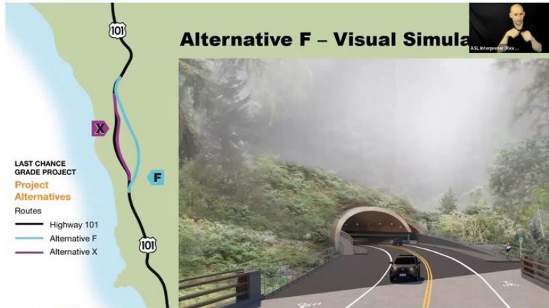
A 6,000 foot tunnel is one of two options Caltrans is considering for a bypass around Last Chance Grade. | Visual simulation courtesy of Caltrans District 1
